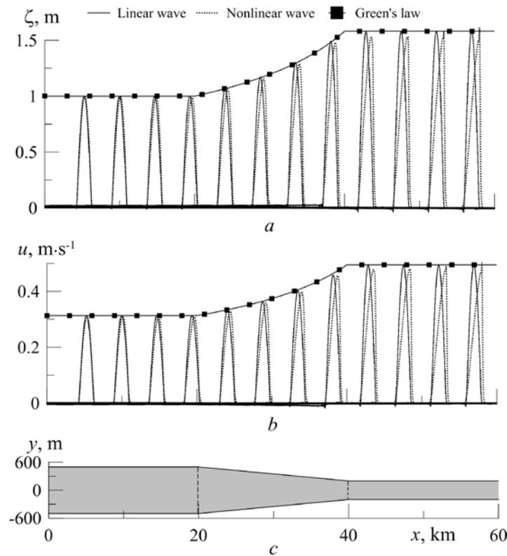
**Fig. 4.** Transformation of the wave form (a) and the horizontal velocity distribution (b) with time for a narrowing channel (c) at decrease of its width from 1000 to 400 m
