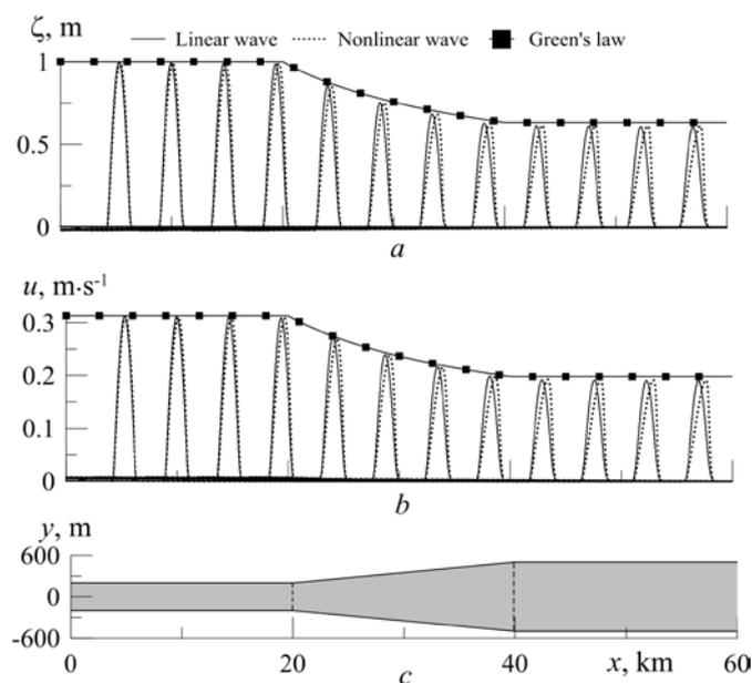
**Fig. 3.** Transformation of the wave form (*a*) and the horizontal velocity distribution (*b*) with time for a widening channel (*c*) at increase of its width from 400 to 1000 m. The channel depth is constant and equals 100 m, the wavelength is 2 km
