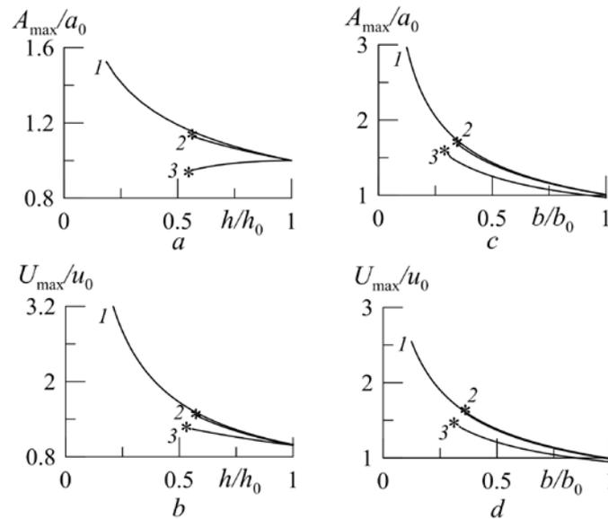
**Fig. 6.** Dependences of the dimensionless wave amplitudes  $A_{\max}/a_0$  ( $a, c$ ) and dimensionless wave velocities  $U_{\max}/u_0$  ( $b, d$ ) upon the basin depth  $h/h_0$  ( $a, b$ ) and the channel width  $b/b_0$  ( $c, d$ ) at constant depth 100 m for linear (curves 1) and non-linear (curves 2) waves, and also at taking into account bottom friction (curves 3)
