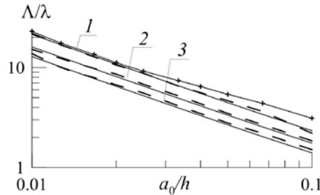
**Fig. 5.** Dependences of the distance related to the initial wavelength ( $\Lambda/\lambda$ ) and traversed by a non-linear wave up to its breaking, upon the non-linearity parameter  $a_0/h$  for different forms of the channel cross-section: 1 – at  $m = +\infty$ ; 2 – at  $m = 2$ ; 3 – at  $m = 1$  (dash line denotes numerical estimates, solid line – analytical estimates, crosses – numerical estimates taking into account bottom friction)
