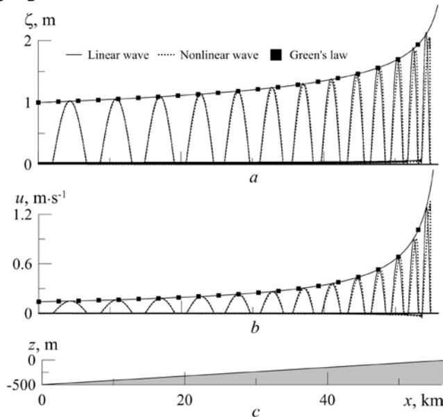
**Fig. 2.** Transformation of the wave form (a) and the horizontal velocity distribution (b) with time in the zone over the sloping bottom (c). The initial wave height is 1 m, the wavelength is 5 km
