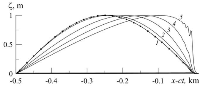
**Fig. 1.** Evolution of a single surface wave (the initial height is 1 m and the wavelength is 0.5 km) in the basin of 25 m depth: curve 1 is a linear wave; curves 2 – 5 are the non-linear waves at the time moments 30, 60, 90, 120 sec, respectively
