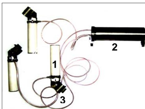
**Fig. 13.** A suspension collection module (trap) consists of: 1 – storage glass; 2 – signal processing unit; 3 – glass fitting
