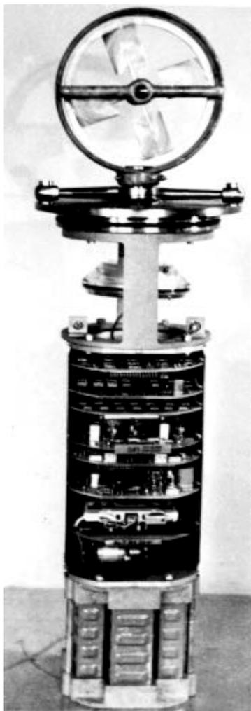
**Fig.4** The long-term component current recorder
