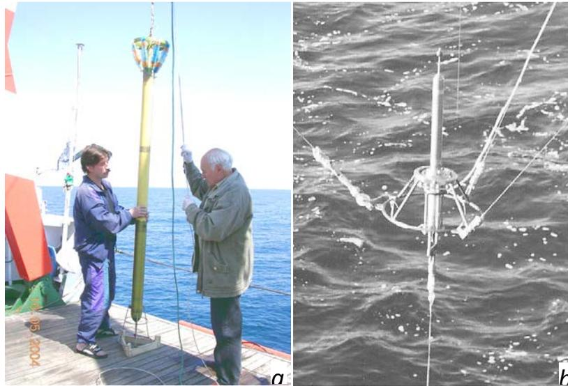
**Fig. 15.** Works with the complex “Sigma” probing variant in the international expedition on the Bulgarian R/V *Akademik* – *a*; co-complex “Sigma-P” (stationary variant) on the oceanographic platform in Katsiveli – *b*
