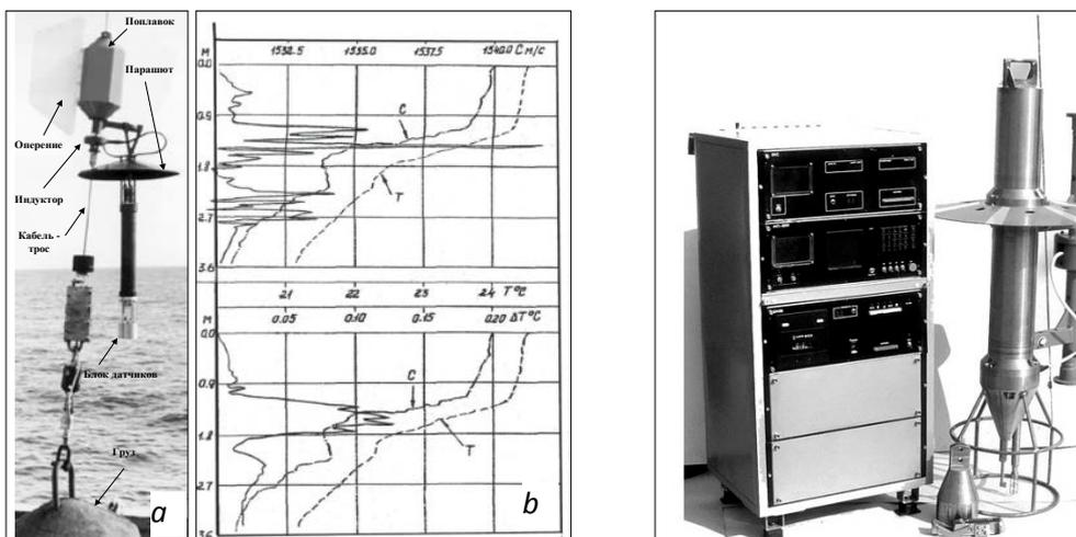
**Fig. 5.** *Zond-ST* falling along the cable rope – *a*; temperature and sound velocity profiles, their vertical gradients and the transient layer in the Black Sea in summer – *b*
