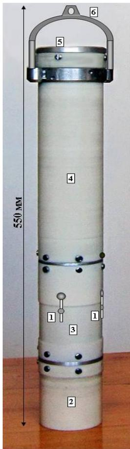
**Fig. 16.** Autonomous electromagnetic current meter: 1 – two of the four electrodes; 2 – false case with the load; 3 – sensor compartment; 4 – electronics and battery compartment; 5 – cover; 6 – suspension handle
