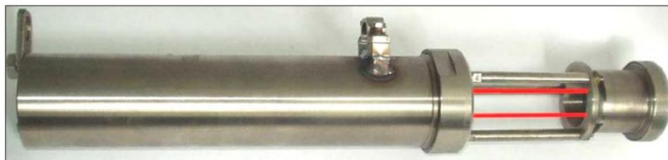
**Fig. 12.** Directional attenuation coefficient meter (transparency meter)
