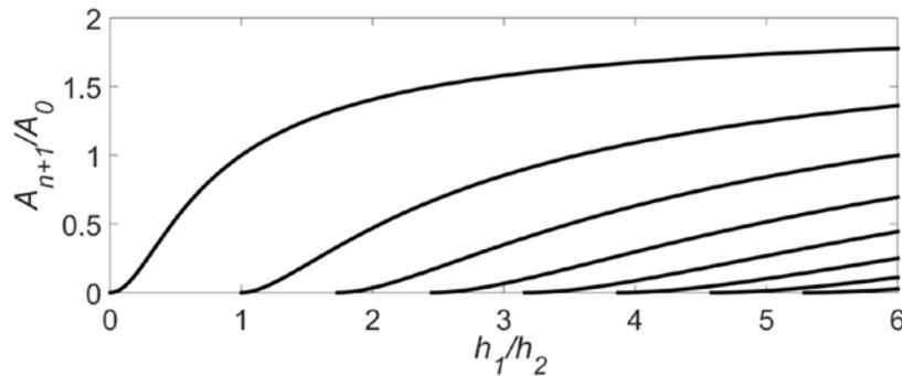
Fig. 2. Dependence of generated soliton amplitude on depth changes
