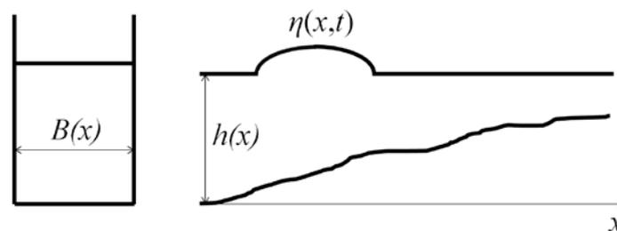
**Fig. 1.** Channel geometry: *on the left* – transversal projection, *on the right* – longitudinal projection
