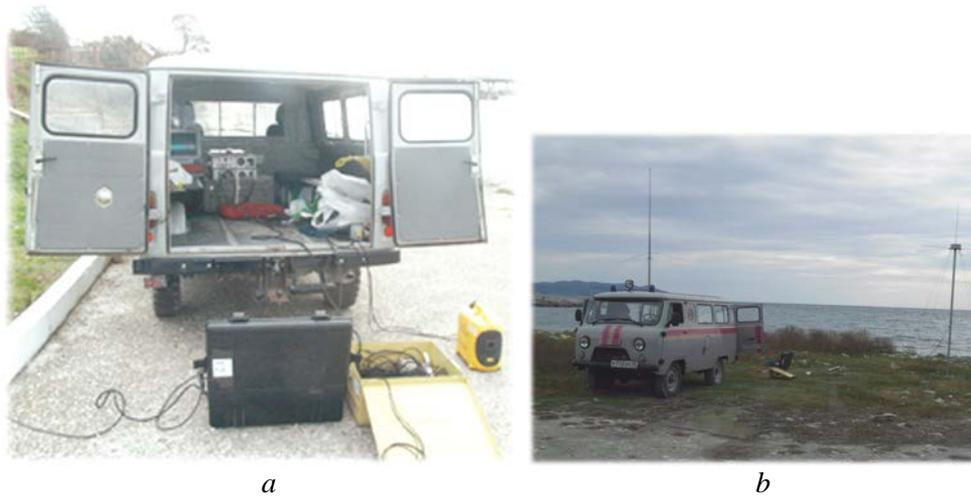
**Fig. 1.** Layout of the measuring equipment in the minibus (*a*) and the position pattern of the radar antennas on the shoreline (*b*)
