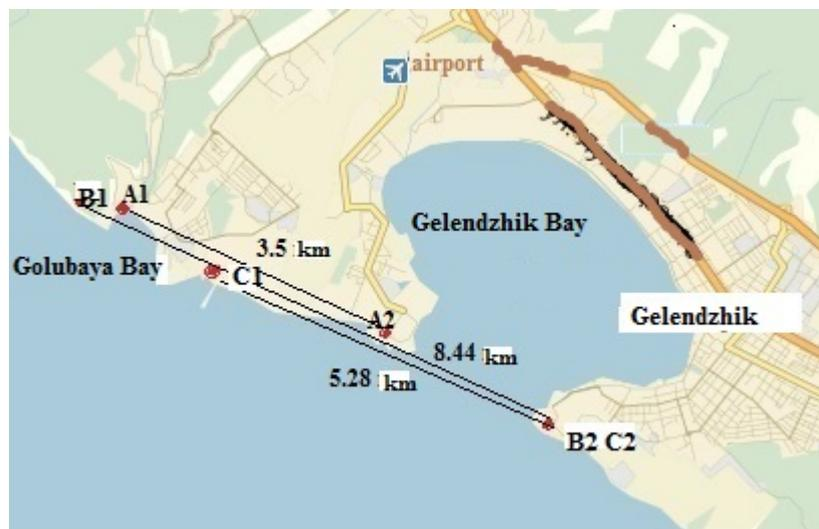
**Fig. 2.** Position of the radar antenna installation points on the shoreline during the measurements in October, 19–21. A1 and A2 points – for October, 19, B1 and B2 points for October, 20 and C1 and C2 points for October, 21
