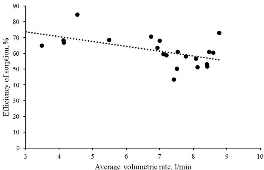
**Fig. 2.** Dependence of the  $^{137}\text{Cs}$  recovery rate on the average volumetric seawater flow rate
