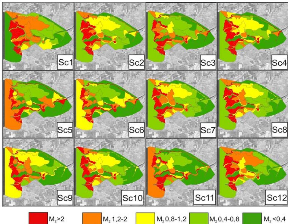
**Fig. 2.** Spatial distribution of the sediment accumulation index over 2 days of calculations ( $M_2$ ) at various combinations of the Don water flow content, reed surface roughness and surge heights
