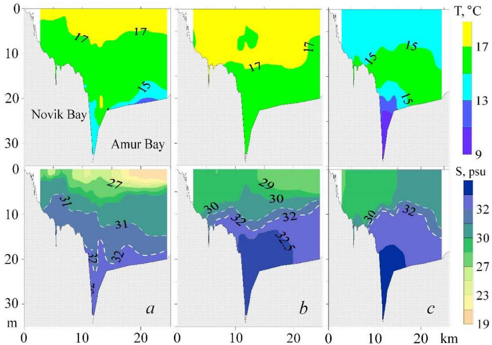
**Fig. 3.** Temperature ( $T$ ) and salinity ( $S$ ) at the axial section NA measured by the XR-620 probe on September, 8 (*a*), September, 29 (*b*) and October, 11 (*c*), 2016
