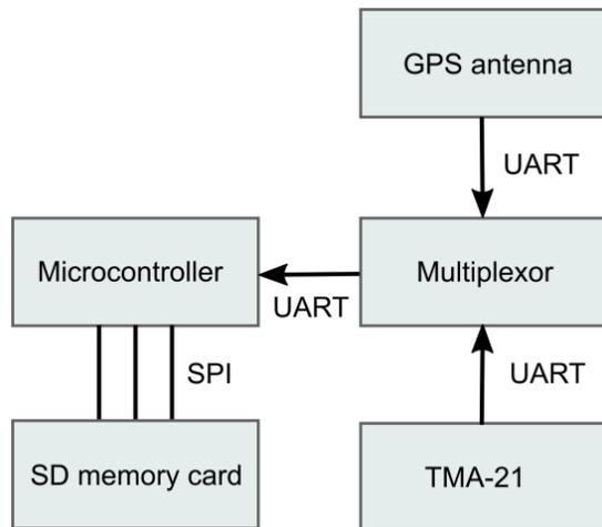
**Fig. 3.** Overview of USV (*a*) and functional scheme of the TMA-21 conductometer converter (*b*). UART – Universal Asynchronous Receiver and Transmitter, SPI – serial peripheral interface
