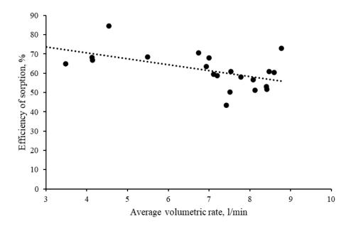
**F i g. 2.** Dependence of the <sup>137</sup>Cs recovery rate on the average volumetric seawater flow rate
