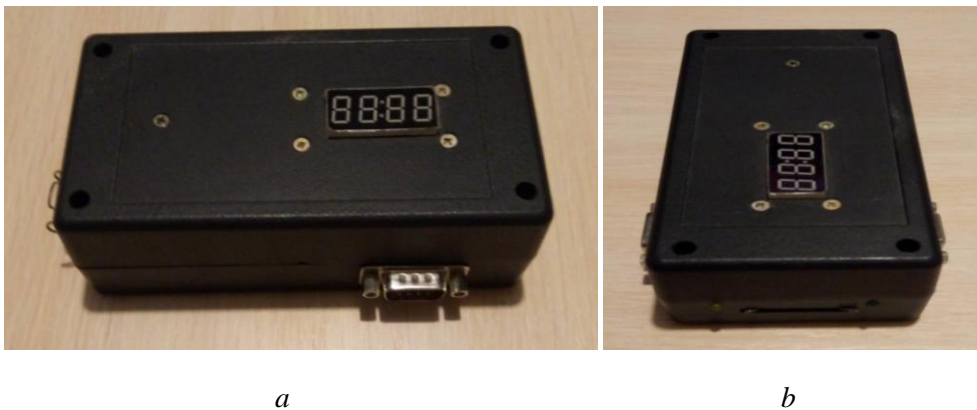
Fig. 7. Appearance of the device for data recording and storing for a single-string wave gauge recorder
