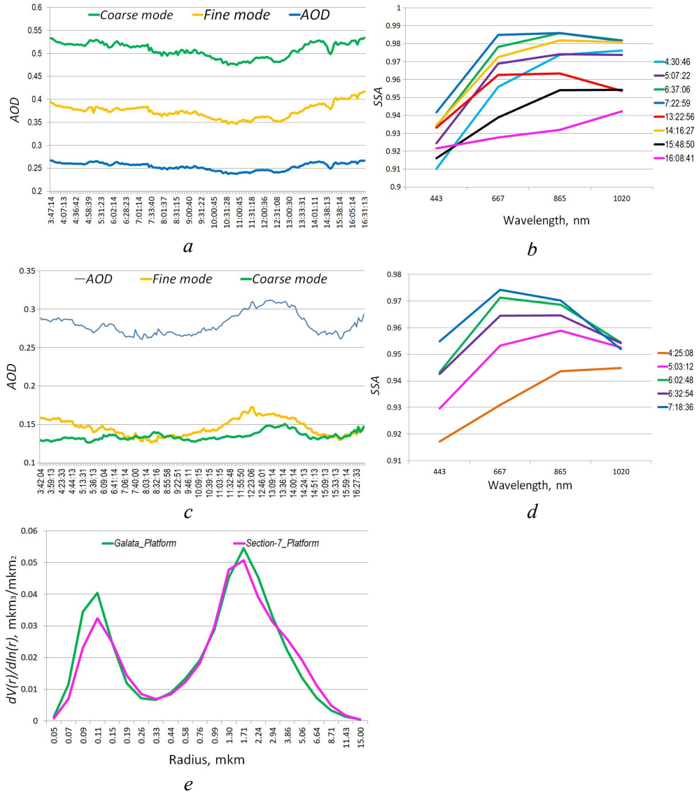
Fig. 2. At the AERONET network stations on 28 July 2021: contribution of fine (less than 2.5 mkm) and coarse particles (2.5 mkm and more) to the overall distribution of AOD at Galata_Platform (a) and Section_7 (c), single scattering albedo at Galata_Platform (b) and Section_7 (d), particle size distribution at two stations (e)
