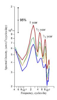
**F i g. 2.** Density spectra of the kinetic energy oscillations of the coastal current within the range 75 days - 6 years at the 5, 10, 15 and 20 m horizons (red, green, orange and blue lines, respectively) at the 95% confidential interval
