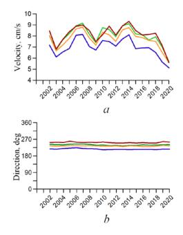
**F i g. 1.** Chronological realizations of variability (2002–2020) of the average annual values of velocity module (*a*) and direction (*b*) of the coastal current at the 5, 10, 15 and 20 m horizons (red, green, orange and blue lines, respectively)
