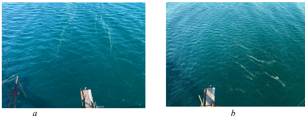
Fig. 3. Langmuir bands at the SOP visualised using wood shavings and sawdust: a – at 17:53 on 20.08.2024, at V_{10} = 10 m/s; b – at 18:57 on 20.08.2024, at V_{10} = 5 m/s
