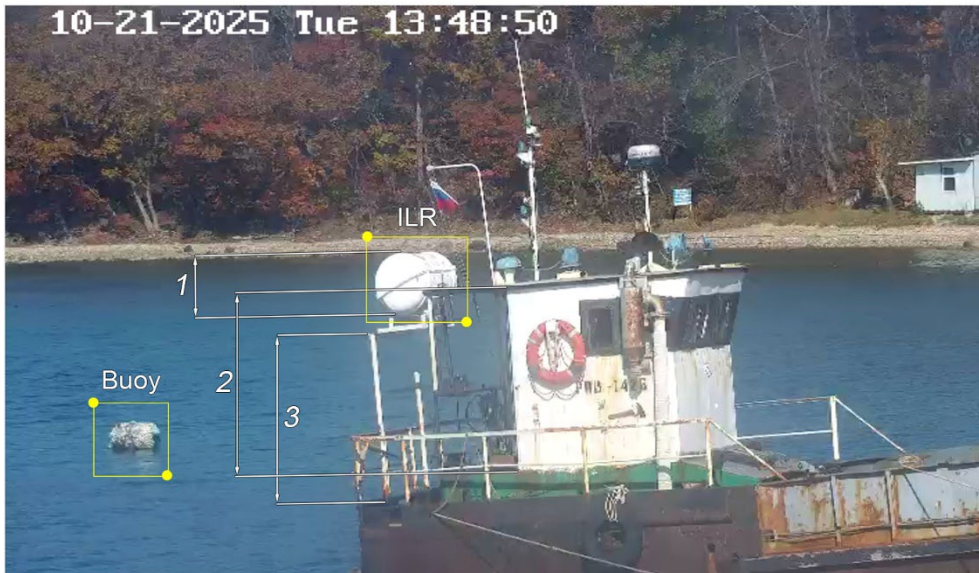
Fig. 2. Frame from continuous video recording of marker objects in Alekseev Bay, showing the elements used for metric image calibration: 1 – diameter of the inflatable life raft (ILR); 2 – edge of the deckhouse structure; 3 – the left vertical post
